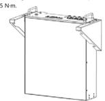
4.Meanwhile, two or four batteries could be installed by theses brackets.
