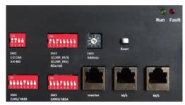
SW1: For CAN communication, please set pin1 and pin2 at on, pin3 and pin4 at off For 485 communication, please set pin1 and pin2 at off, pin3 and pin4 at on SW4,SW5: Please use them to set the port of RJ45
