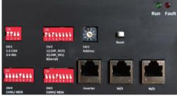
SW1: For CAN communication, please set pin1 and pin2 at on, pin3 and pin4 at off For 485 communication, please set pin1 and pin2 at off, pin3 and pin4 at on SW4,SW5: Please use them to set the port of RJ45
