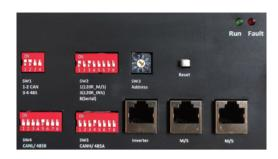
Please make sure the SW2 DIP switch selected correctly, if the battery connected in Parallel mode, but select SW2 DIP8 at ON position, probably lead serious fault even dangerous. Meanwhile, if battery connected in Series mode select SW2 DIP8 at OFF status, serious fault and dangerous probably occurred.
